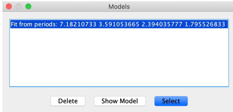
Models can be deleted or selected for plotting or inspection. Clicking the Show Model button opens a dialog that shows the selected model function in different forms.
