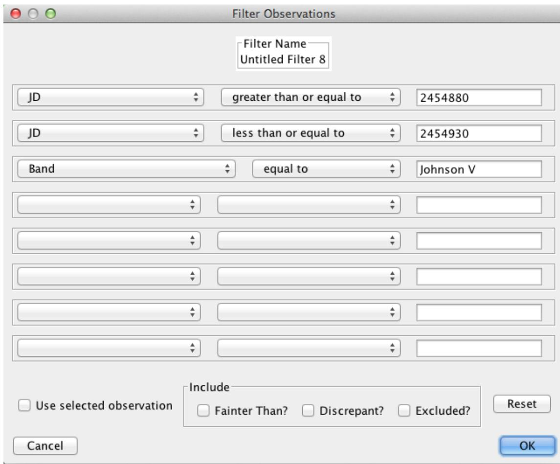
Note that the “Filter Name” text box at the top of the observation filter dialog can be modified to give a filter a meaningful name, e.g. “2454880...2454930 V.”
