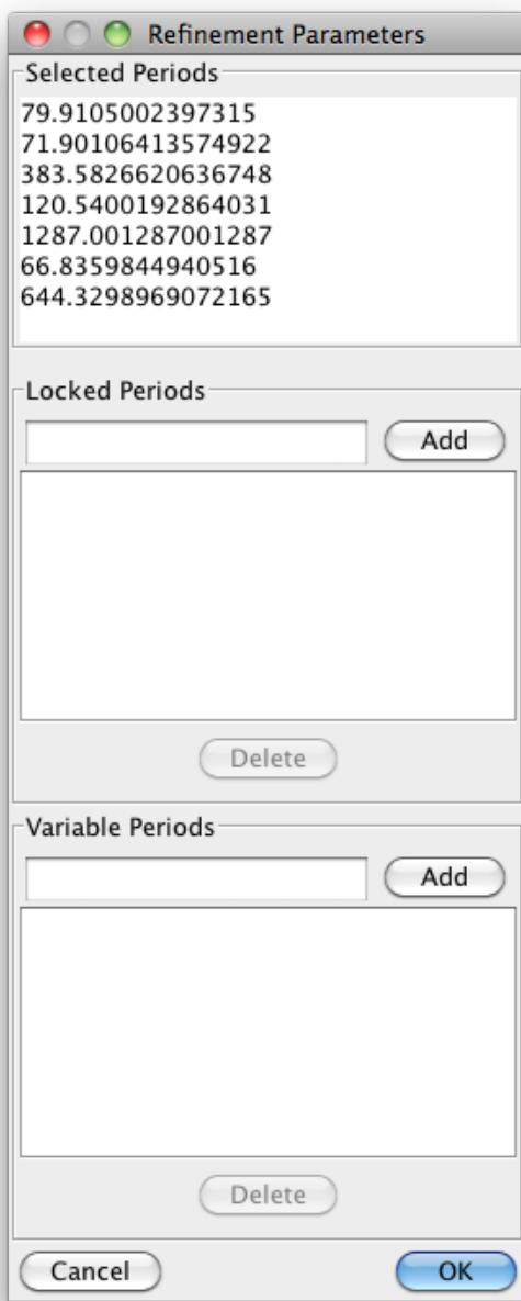
Clicking OK here adds seven new top hits with the same power value, shown multiply-selected in the top hits list and annotated on the power spectrum.
