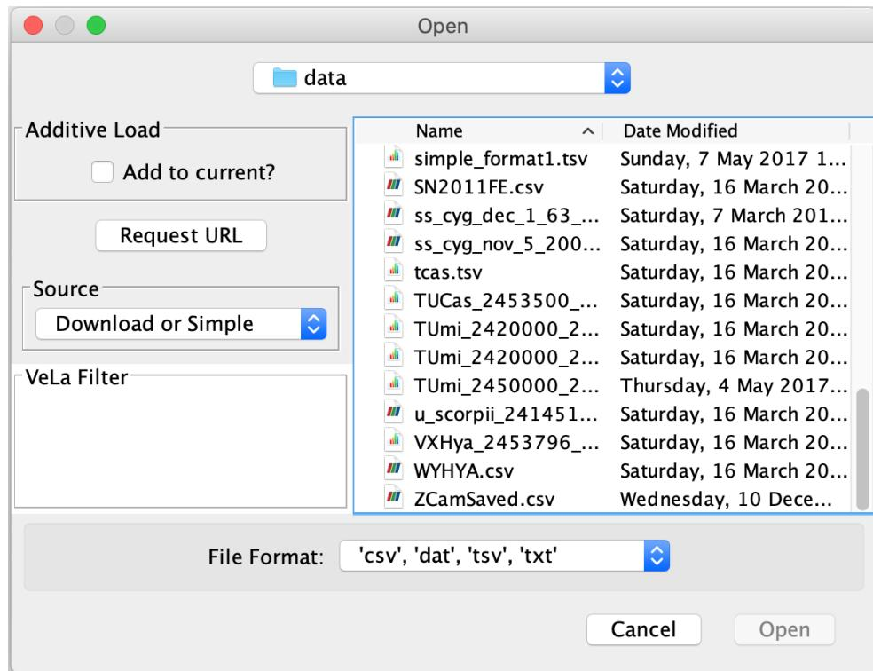
Choosing a conformant file and clicking the Open button will load the observations, leading to the same result as a Load from AID operation. If the file is not of a suitable format, an error dialog will be displayed.
